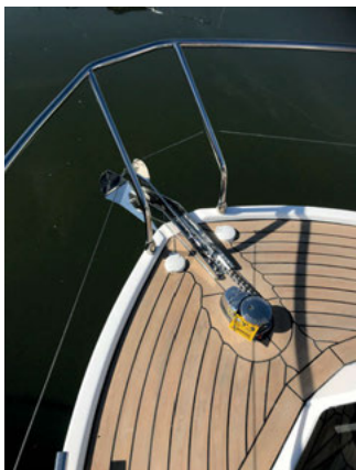
Substantial ground tackle includes a stainless steel plough anchor and a chain and electric winch operated by foot switches.
